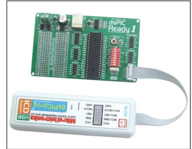
Figure 1-2: *dsPICflash* connected to the *dsPIC Ready1* board
