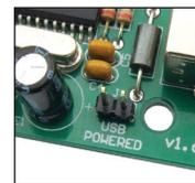
Figure 1-5: The *dsPICflash* programmer is powered from the target device supplied with the microcontroller.
