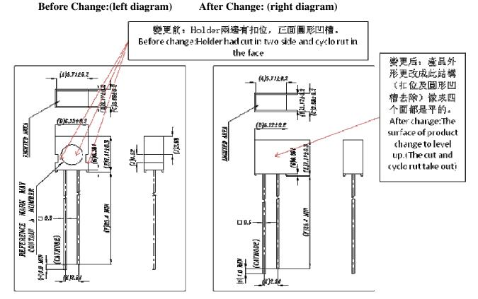
備註:除上述Holder兩邊有扣位,正面圓形凹槽變更外,其它尺寸不變。 PS:All other dimensions may remain, beside the The cut and cyclo rut taking out.
