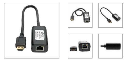
Works with Tripp Lite's B126-Series transmitters to extend an HDMI signal via Cat5e/6 cable up to 100 ft. to a projector, monitor or television. Ideal for digital signs, schools and trade show presentations.
