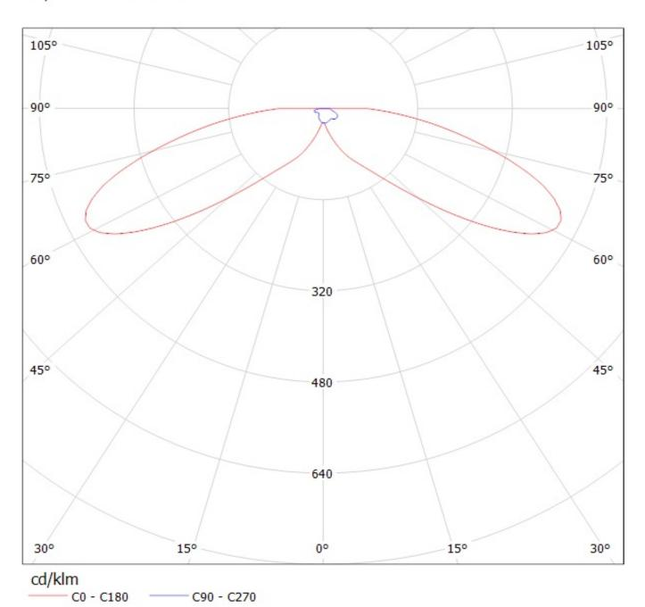
Luminaire: LEDiL Oy CA11892\_STRADA-SQ-T-DW\_(XP-G2) Eff: 93% Lamps: 1 x CREE\_XP-G2\_(XPGBWT-H1-7B4-R4-0-04)\_106.35Im@250mA\_P=0.755748W\_I=249.9mA
