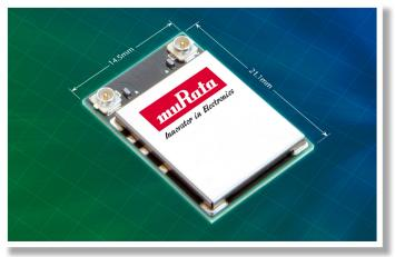
The SN1857 provides 2.4 and 5 GHz WLAN plus Bluetooth and NFC functionality in a small, FCC/IC certified and ETSI compliant module. The SN1857 is based on TI's WL1857 SOC.
