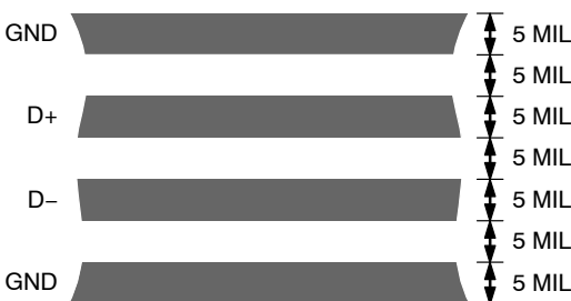
Figure 21. Typical Arrangement of Signal Tracks
