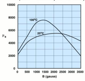
Measured on an 18/10/6mm toroid at 10kHz.
