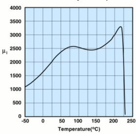
Measured on an 18/10/6mm toroid at 100kHz.
