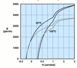
Measured on an 18/10/6mm toroid at 10kHz.
